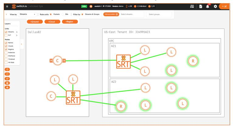
Configuration is as simple as selecting a source and adding destinations. All eligible SRT listeners are highlighted. Selecting any of them completes the SRT connection.
